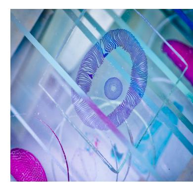
The Rogers lab developed a biocompatible skinlike sensor for continuous monitoring. They have focused on devices that can be adhered to the skin, but in the future, envision them being used directly with organs such as the heart and the brain. His work is based on adapting the electronic engineering found within consumer devices to interface with the soft tissues of the human body.
