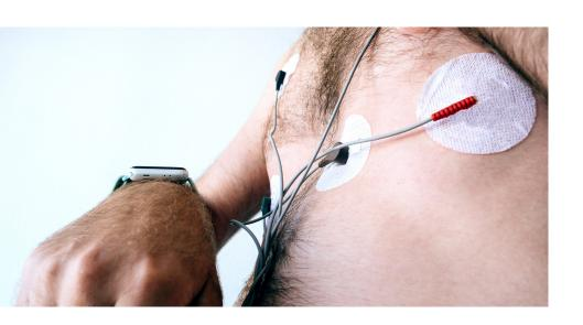
The idea is to develop a wireless platform, eliminating the forces imparted through the wires to the interface between the biosensors and the skin. We would use an adhesive strength with a factor of 10 or 100 times lower than that, which is required for the wired based devices. The consequence of that is that you end up with a much more comfortable interface with less skin irritation.
