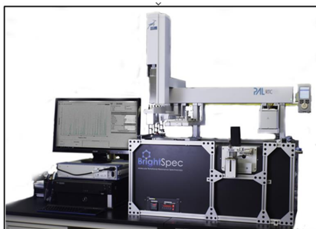
Figure 1. A picture of the BrightSpec-ONE spectrometer. Default sampling options include the online-capable gas flow inlet (GFI) and direct injection port (DIP). Additional sampling and automation options include static headspace sampling module (HSM) and PAL-RTC autosampler for analysis of volatile impurities in solutions and solids.
