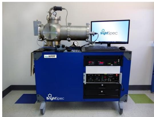
**Figure 1.** A picture of a commercial isoMRR™ unit capable of quantitative analysis of impurities in complex chemical mixtures including regioisomers, diastereomers, enantiomers, and isotopomers. Instrument is equipped with online-capable sampling manifold.
