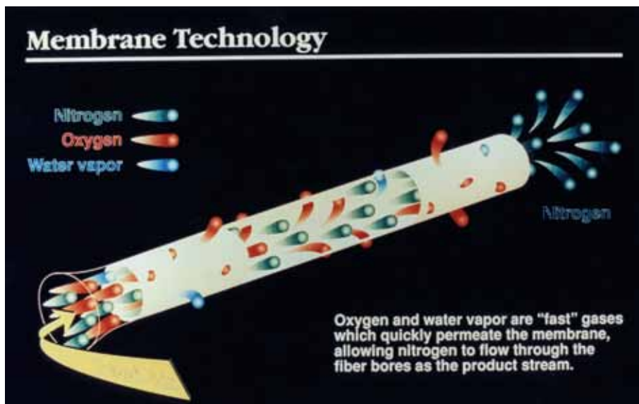
Figure 1: Hollow fiber membrane bundle separates nitrogen from air. Oxygen and water vapor permeate the membrane, allowing nitrogen to flow through the tubes.
